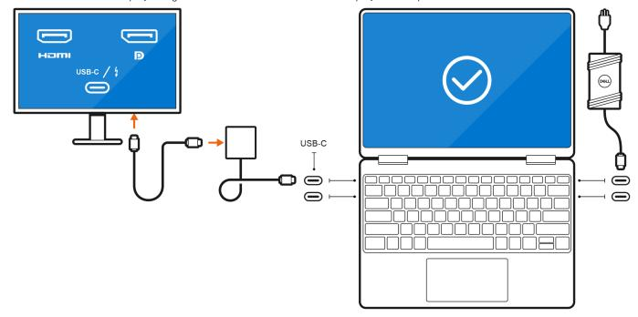
• Connect up to two external displays using a USB-C docking station:
